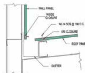
VALLEY GUTTER AT HIGH-LOW ROOF TRANSITION
