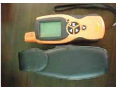
Dewmeter/Humid 20% ~ 99% / Temp. 0°C ~ 50°C
