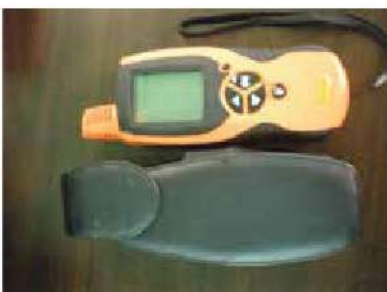
Dewmeter/Humid 20% ~ 99% / Temp. 0°C ~ 50°C
